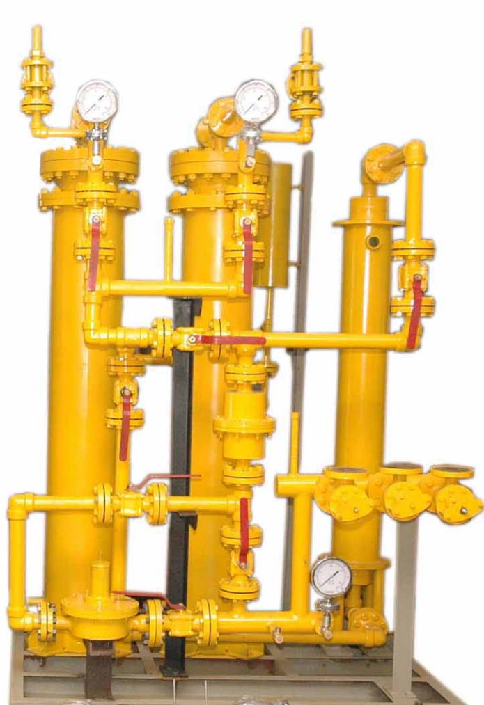
LIQUID (CL 2 ) CHLORINE VAPOURIZER SYSTEM AND CONTROLS 1000 Kg/h
